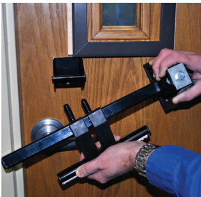
Place hooks on quick release bracket. Allows responders to unlock with security key.
